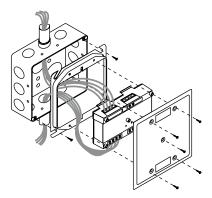
**SIGA-MRM1:** mount the UIOxR motherboard inside a suitable EDWARDS enclosure with screws and washers provided. Plug the module into any available position on the motherboard and secure the module to the motherboard with the captive screws. Wiring connections are made to the terminals on the motherboard (see wiring diagram). UIOxR motherboard terminals are suited for #12 to #18 AWG (2.5 mm2 to 0.75 mm2) wire size.
